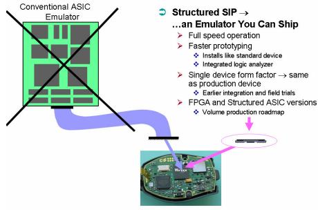
be incorporated into the final form factor of the customer's product, which delays much of the testing that comes from field trials. Structured SIP devices fit the same footprint as the final production ASIC, and can be used in the final form factor of the ASIC developer's product.
