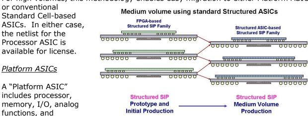
uncommitted logic constructed on the same die where the device can be customized with only a few custom masks. The uncommitted logic fabric is constructed with a "Structured ASIC" type of architecture, enabling much faster development, and a lower prototype cost due to significantly lowered mask costs.
