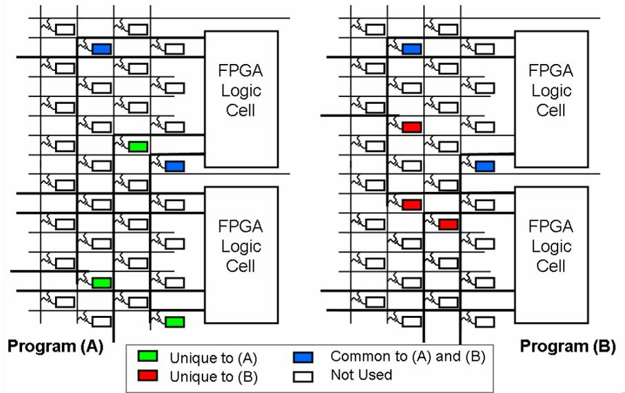
implementations of the conventional FPGA as shown in this figure, we notice that some switches are only turned on for program A (green), some only turned on for program B (red), and a few turned on for both programs A and B (blue).
