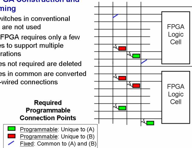
The physical implementation for this hybrid architecture can be constructed in more than one manner. First of all, custom silicon can be constructed using standard cell or full custom techniques, and for some applications this may be the best choice. In most applications, however, it may be more prudent to implement the hybrid FPGA architecture using Structured ASIC techniques. Structured ASIC's are configured with a
