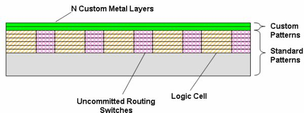
Shown here using Structured ASIC techniques
