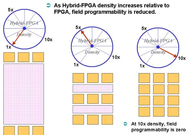
at a particular application segment, and also retains a (lesser) degree of field programmability, the remaining programmability being focused within that segment to allow for changes.
