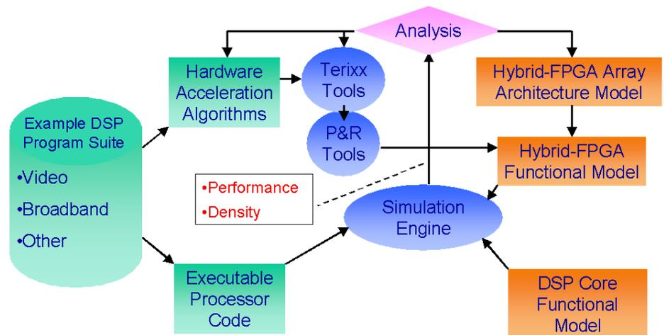
In the case of the Hybrid-FPGA fabric for an rDSP device or any embedded (ASIC) application, the simulation should include a composite of both hardware simulation for functions within the Hybrid-FPGA as well as simulation of the software running on the processor including the interaction of the two.
